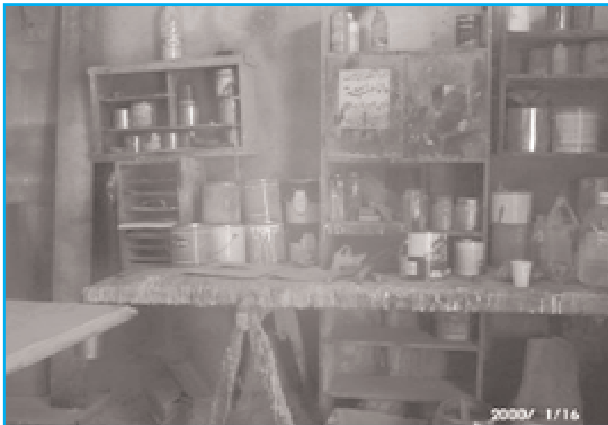
Photo 12: Chemicals are haphazardly stored. This is a potential risk to workers health in their working environment.
