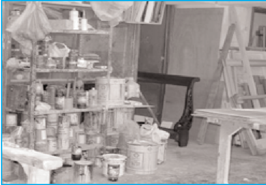
Photo 13: Chemicals are haphazardly stored. This is a potential risk to workers health in their working environment.
