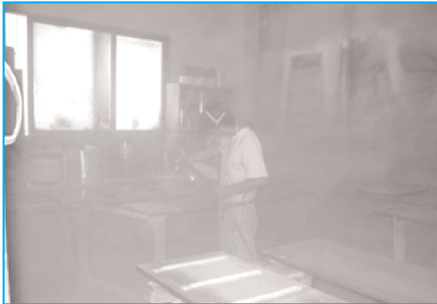
Photo 9: The haze in the photo is a definite proof of the absence of adequate ventilation for the protection of the worker. The airborne chemical may have the capacity to penetrate through skin and therefore the worker is by no means fully protected.
