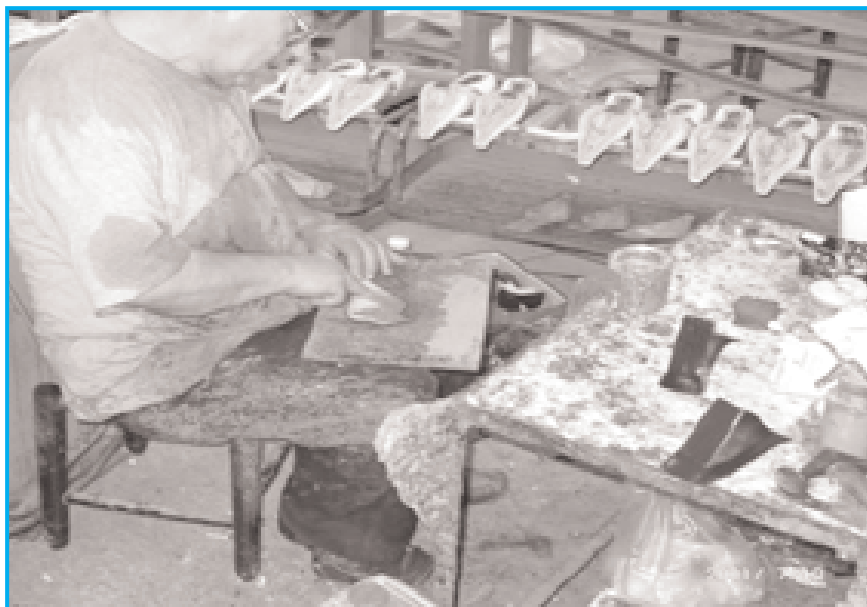
Photo 2: Gluing with fingers, and using pastes to wipe fingers, thus potentially increasing chemicals through direct or indirect skin contamination.
